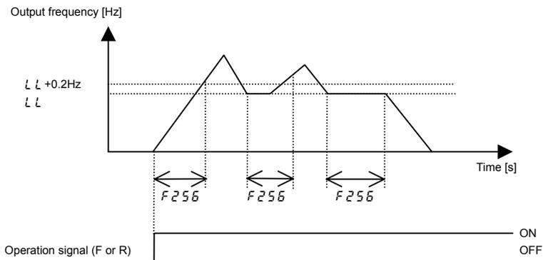
Note: This function is enabled even at the start of operation and during switching between forward and reverse run.
