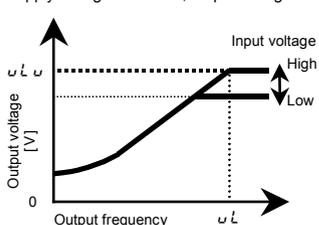
[2: Supply voltage uncorrected, output voltage unlimited]
