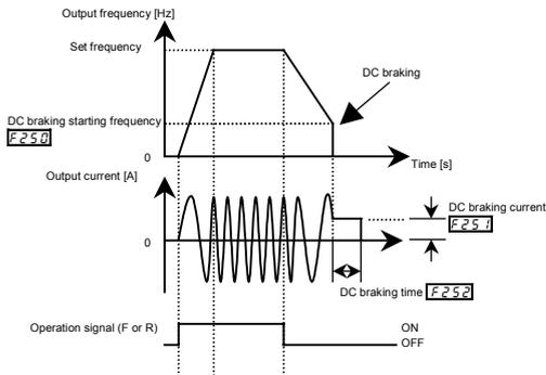
Note 1: During DC braking, the overload protection sensitivity of the inverter increases. The DC braking current may be adjusted automatically to prevent tripping.
