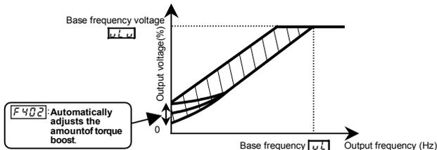
Note: This control system can oscillate and destabilize runs depending on the load. If that should happen, set V/F control mode selection  $P\text{L}2$  to  $0$  (V/F constant) and increase torque manually.
