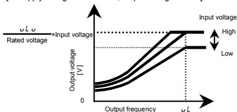
\* The above applies when V/F control mode selection parameter  $P\omega$  is set to "0" or "1".
