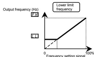
\* The output frequency cannot be set at less than  $LL$ .
