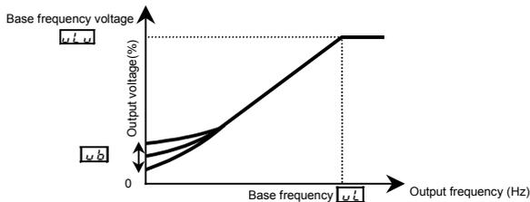
\* To increase the torque further, increase the setting value of the manual torque boost  $u\ b$ .
