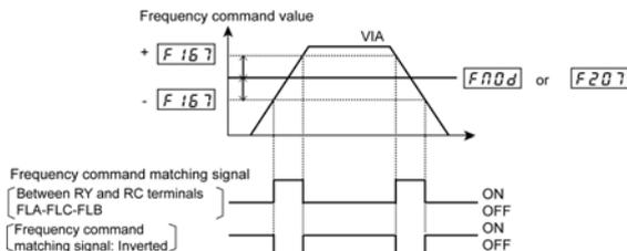
Note: This function can be used, for example, to send out a signal indicating whether the amount of processing and the amount of feedback agree with each other when the PID function is in use.
