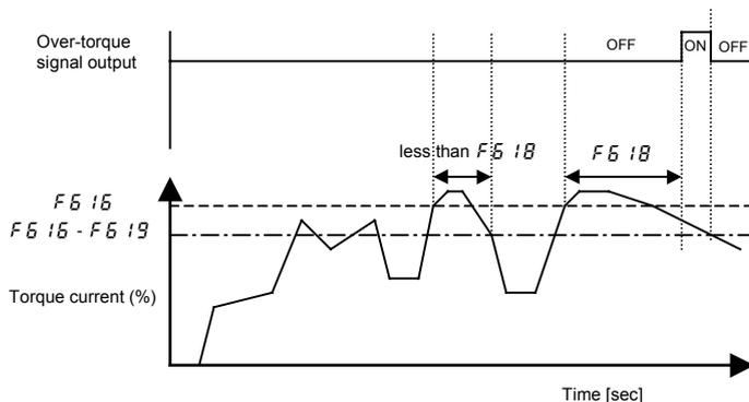
When  $F\delta 15 = 1$  (tripping), the inverter will trip if over-torque lasts for the period of time set with  $F\delta 18$ . In such a case, the over-torque signal remains ON.
