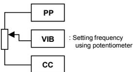
\* The input terminal VIA can be used in the same way.
