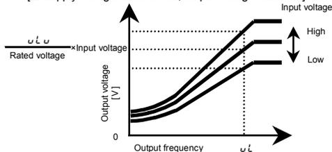
\* The above applies when V/F control mode selection parameter  $P\omega$  is set to "0" or "1".
