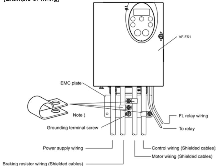
Note: Strip and earth the shielded cable, following the example shown in Fig.
