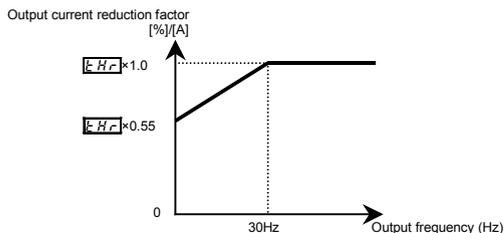
Note: The motor overload protection start level is fixed at 30Hz.
