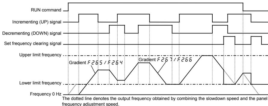
Note: If the operation frequency is set to the lower limit frequency, it will increase from 0Hz when power is turned on for the first time after the setting, and therefore the output frequency will not rise until the operation frequency reaches the lower limit frequency. (Operation at the lower limit frequency)
