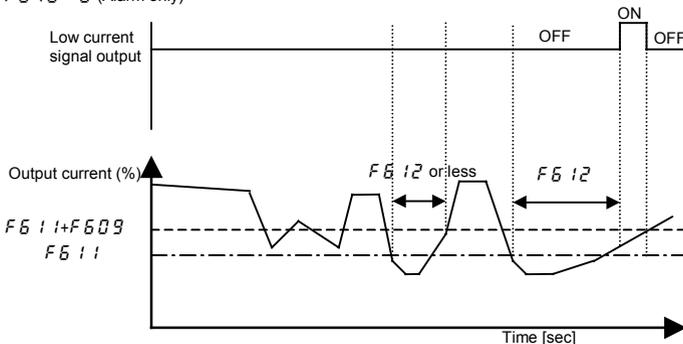
\* When setting *F510* to 1 (Trip), trip after low current detection time setting of *F512*. After tripping, the low current signal remains ON.
