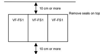
The space shown in the diagram is the minimum allowable space. Because air cooled equipment has cooling fans built in on the top or bottom surfaces, make the space on top and bottom as large as possible to allow for air passage.
