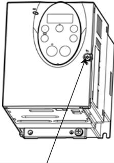
Turn the locking screw on the right side of the front panel 90° counterclockwise to align the dot on the screw with the unlock position mark (upper side). To avoid damage to the screw, do not apply excessive force to turn the screw more than 90 degrees.
