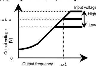
\* Even if  $\omega L \omega$  is set for an output voltage lower than the input voltage, the output voltage will exceed the voltage adjusted by  $\omega L \omega$  when the output frequency is higher than the base frequency  $1 \omega L$ .
