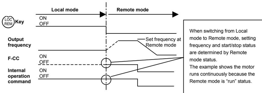
To prevent from moving the setting frequency and start/stop status of Remote mode to Local mode, the F 2 9 5 is set to "0"(Disabled). In this case,
