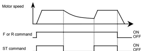
★ Setting  $F3Q1$  to 2 or 3: This function operates after the ST terminal connection has been OFF first and then ON again.
