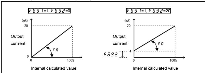
Note 1: When using the FM terminal for current output, be sure that the external load resistance is less than 750Ω.
