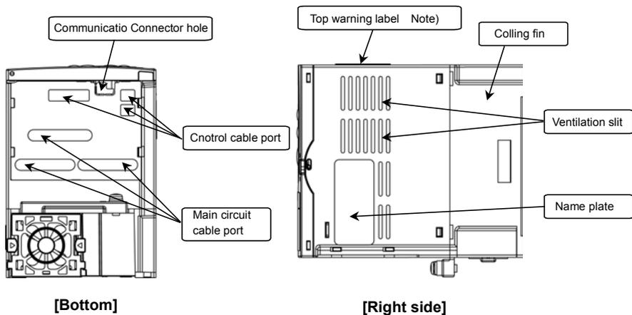
**Note:** Remove this seal and operate it at a current lower than the rated one when installing the inverter side by side with other inverters where the ambient temperature will rise above 40°C.
