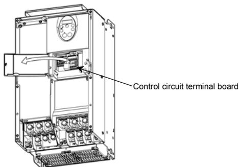
Open the control circuit terminal board cover.
