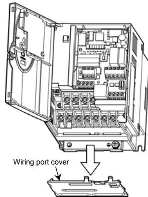
Remove the wiring port cover by pulling it down, pass cables through the wiring port, and connect the cables to the terminal board.
