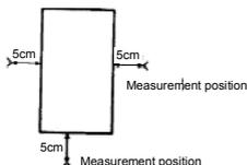
Note: The inverter is a heat-emitting body. Make sure proper space and ventilation is provided when installing in the cabinet. When installing inside a cabinet, we recommend the top seal peeled off although  $40^{\circ}\text{C}$  or less.
