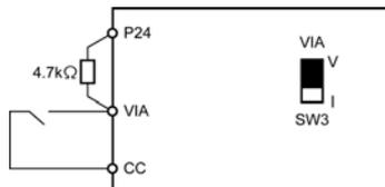
2 ■ Logic switching/Voltage-current output switching (slide switch)
