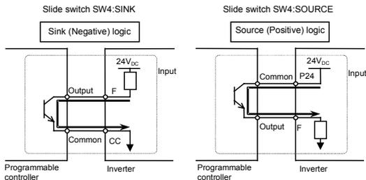
■ SINK (Negative) logic/SOURCE (Positive) logic (When an external power supply is used)
