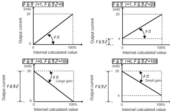
★ The analog output inclination can be adjusted using the parameter  $F\beta$ .
