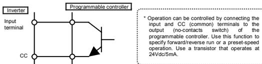
\* Interface between programmable controller and inverter
