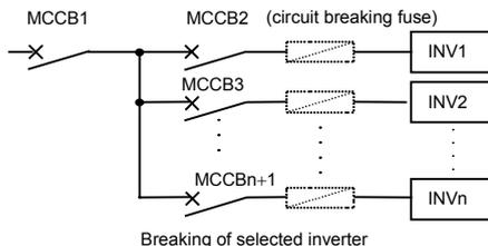
There is no fuse in the inverter's main circuit. Thus, as the diagram above shows, when more than one inverter is used on the same power line, you must select interrupting characteristics so that only the MCCB2 will trip and the MCCB1 will not trip when a short occurs in the inverter (INV1). When you cannot select the proper characteristics install a circuit interrupting fuse between the MCCB2 and the INV1.
