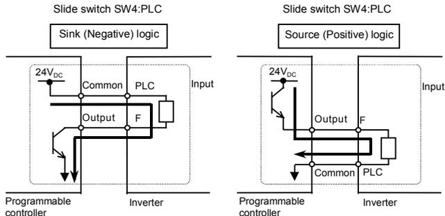
■ Selecting the functions of the VIA terminals between analog input and contact input
