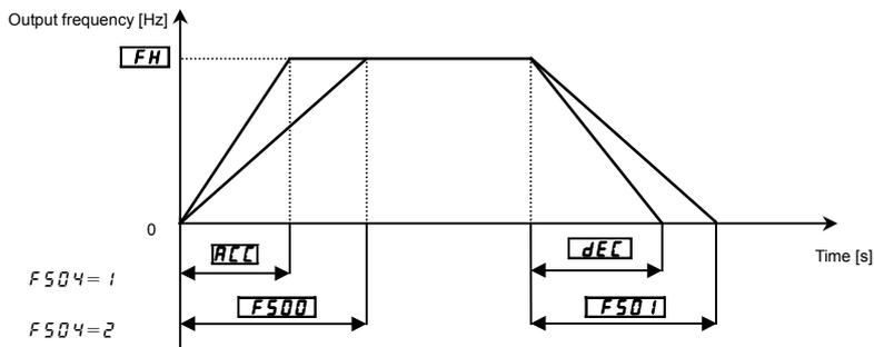
Acceleration/deceleration time 1 is initially set as the default. Acceleration/deceleration time 2 can be selected by changing the setting of the *F504*.
